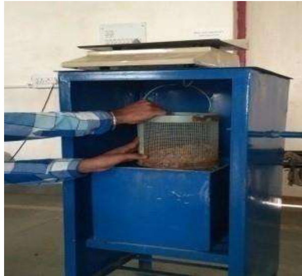
Figure 2 Wire bucket for Specific gravity
