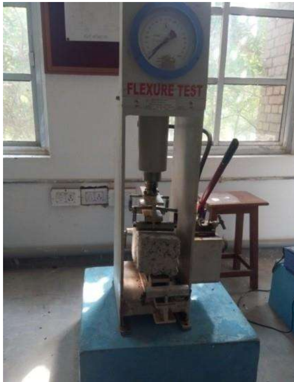
Figure 4 Flexural Strength Test Apparatus
