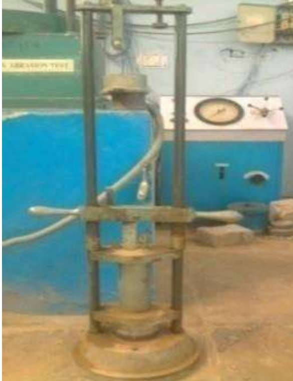
Figure 1 Aggregate Impact Test Machine
