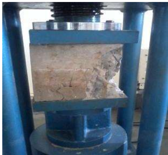
Figure 3 Crushing strength test
