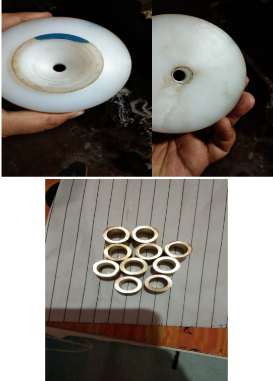
Fig. 2 Fixture top and bottom and brass specimen
