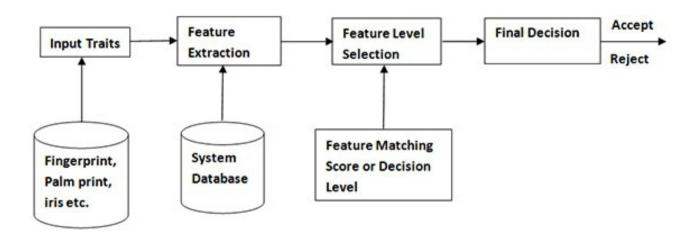
Figure 2: Block diagram of Multimodal Systems Multimodal biometrics provides supplementary information among different modalities in order to increase the recognition performance in terms of accuracy and reliability to overcome the drawbacks of a single biometric system[10].
